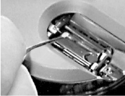
Figure 16-2: Cleaning the sample holder guide bars
