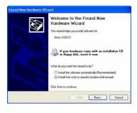
Ensure the Moticam 2300 (MC3001) is plugged into the computer. The "Find New Hardware Wizard" will appear. With the software CD in the CD driver, select "Install the software automatically". If this fails to install the driver, select "Install from a list or specific location (Advanced)", and click "Next".
