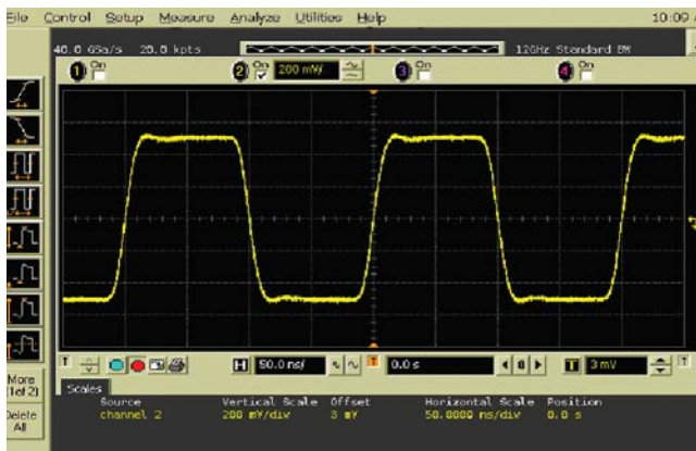
Figure 10. An oscilloscope's voltage versus time display of a square wave
