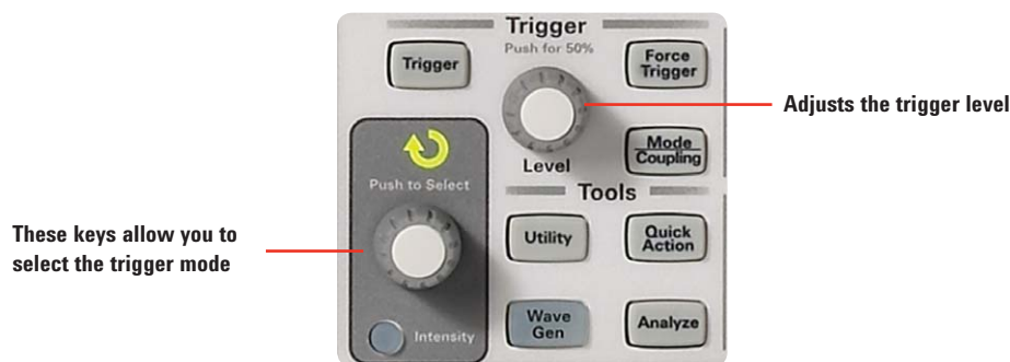
Figure 20. Front panel trigger control section on an Agilent InfiniiVision 2000 X-Series oscilloscope
