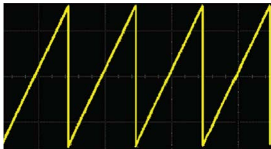
Figure 6. A sawtooth wave
