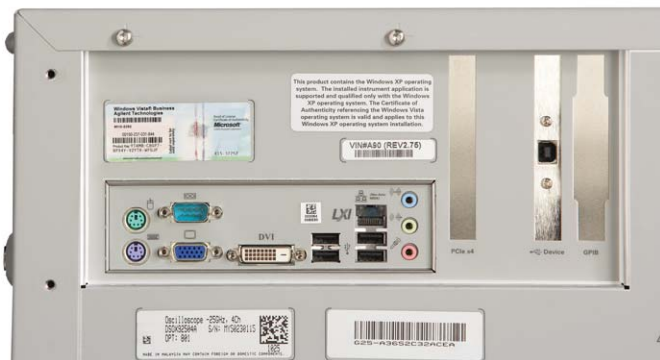
Figure 9. Rear panel on the Agilent Infiniium 9000 Series oscilloscope
